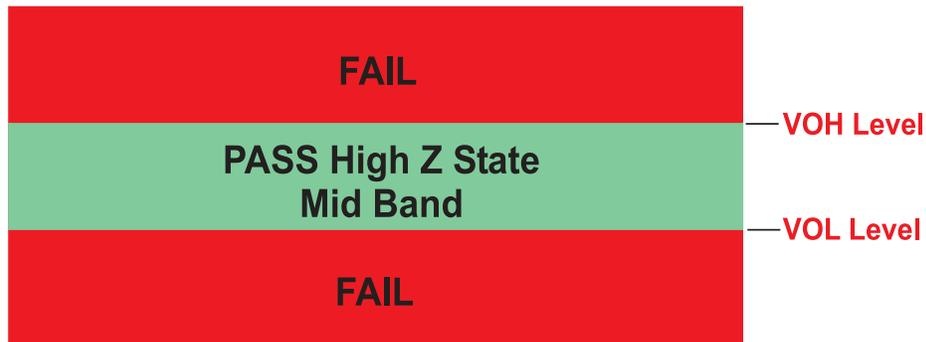
Comparator logic for High Impedance Levels
